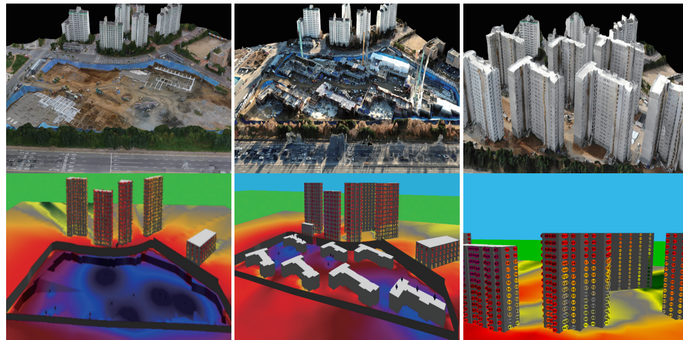
3D Noise Simulation using Photogrammetry
