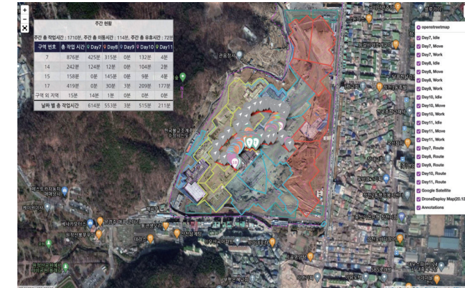
Productivity Analysis Using Heavy Equipment Monitoring System
